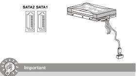
Please do not fold the Serial ATA cable into 90-degree angle. Otherwise, data loss may occur during transmission.
